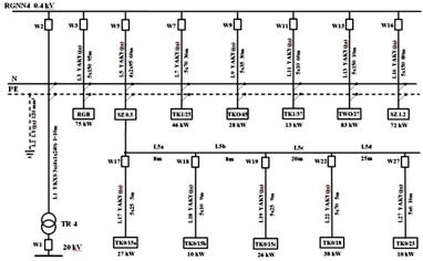
Fig. 3. Simplified scheme of LV electrical network selected for modeling.
