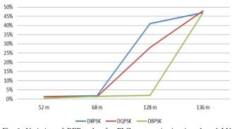
Fig. 6. Variation of BER value for PLC communication in selected LV network structure under 10 % full band noise and with FEC applied.
