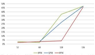
Fig. 8. Variation of BER value for PLC communication in selected LV network structure under influence of 1 kV impulse disturbance with FEC applied.
