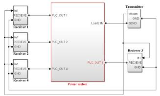
Fig. 5. Block scheme for testing the PLC performance in Mathwork Matlab Simulink.
