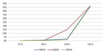
Fig. 7. Variation of BER value for PLC communication in selected LV network structure under 10 % full band noise and without FEC.
