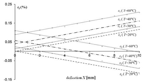
Fig. 6. The relative resistance increments  $J_{1,2}$  in the function of the beam X deflection while temperature T is changing.
