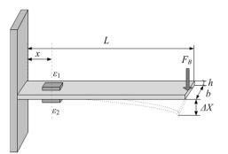
Fig. 4. Two metal strain gauges placed on the cantilever beam. The beam is bent by force  $F_B$  and heated in the same time.
