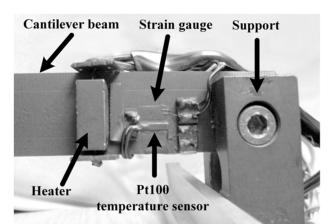
Fig. 7. Localization of heater, RTD sensor and strain gauge.
