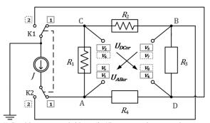
Fig. 1. Double current bridge (2x1J) as an input analog part of measurement system (J-current source,  $R_1$ ,  $R_2$  – sensors,  $R_3$ ,  $R_4$  – resistors, K1, K2 – electronic switches).
