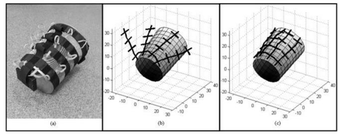
Fig. 5. Test setup (a), reconstruction without and with the described method (b), (c).
