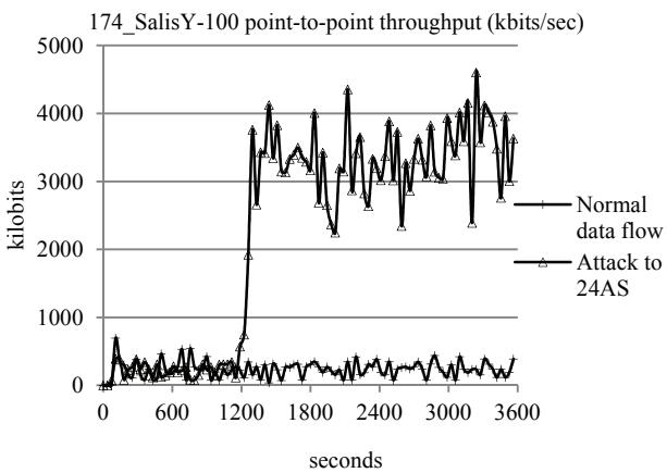
**Fig. 5.** Throughput measurement during the attack scenario 2
