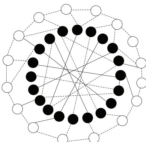
**Fig. 1.** Graph of the state Internet network topology: national AS represented in black nodes; international AS in white; *peering* interconnections type – dotted lines; *transit* – solid lines
