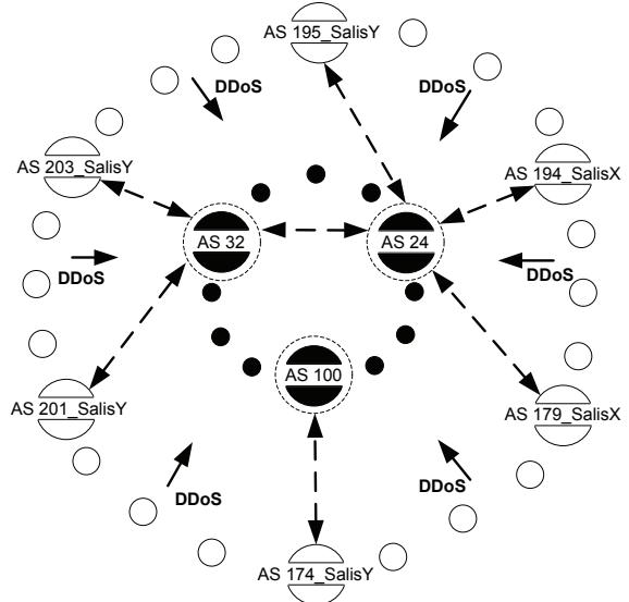
**Fig. 2.** Part of the network topology illustrating type of attack from international AS to the national AS infrastructure (attack vector represented by *DDoS*)
