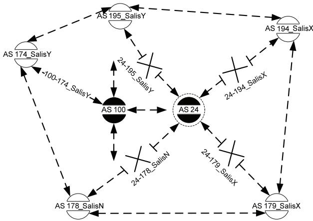
**Fig. 4.** Part of the network topology illustrating the attack on interconnections node (attack vector represented by broken node/lines)
