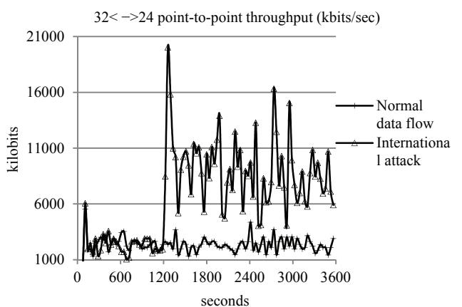
**Fig. 3.** Throughput measurement during the attack scenario 1
