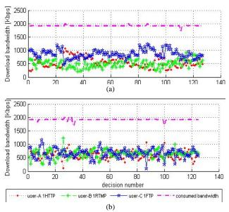
Fig. 3. Example of download bandwidth distribution without (a) and with (b) proposed method.
