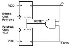
Fig. 4. Typical tri-state PFD block diagram.
