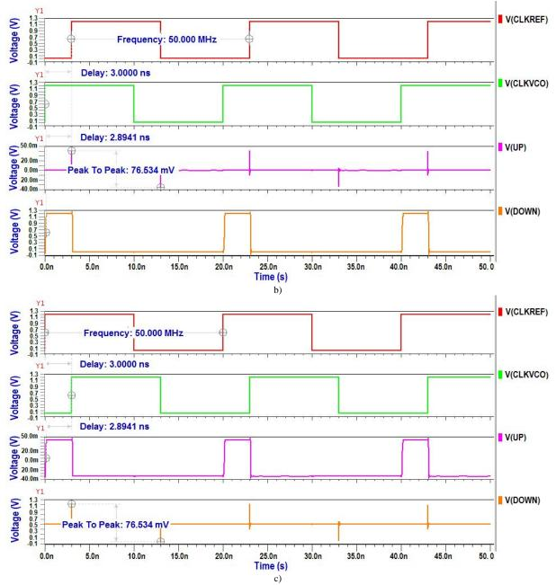
Fig. 6. Modified high speed dynamic PFD output waves for all three conditions.
