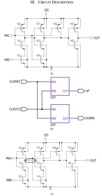
Fig. 5. Utilized UP dynamic schematic with inverter [9] (a), top level schematic of the high speed PFD (b) and modified DOWN dynamic schematic with inverter by [9] (c).
