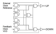
Fig. 3. Conventional logic gates PFD.
