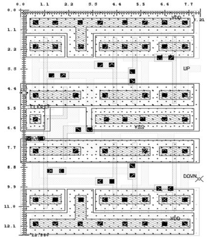
Fig. 8. Modified high speed PFD layout design.
