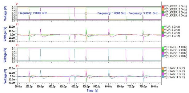
Fig. 7. Modified high speed dynamic PFD operates at matched inputs (locked) in the range of 1 GHz - 4 GHz.
