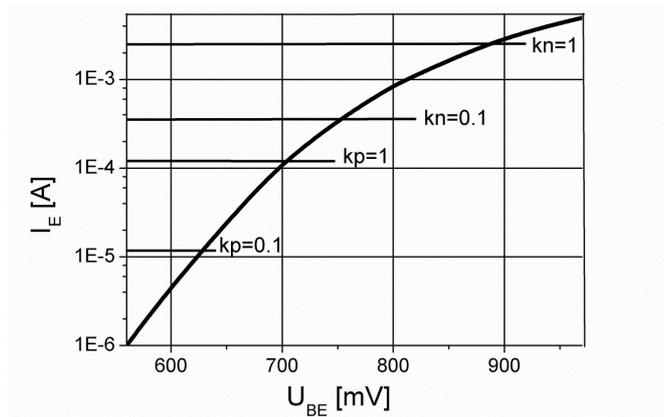
Fig. 2. Experimental voltage-current characteristic of the base-emitter junction of the p-n-p integral lateral transistor with junction area  $1.3 \times 10^{-4} \text{ mm}^2$ .
