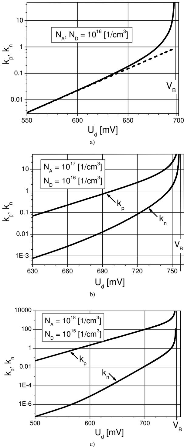
Fig. 1. Dependences of minority carrier hole and electron injection levels on voltage drop across the depletion region for silicon junctions No.1–No.3 calculated using equations (9) and (10) (solid lines). The dependence for junction No.1 presented by the dashed line has been calculated using equations (5) and (6).
