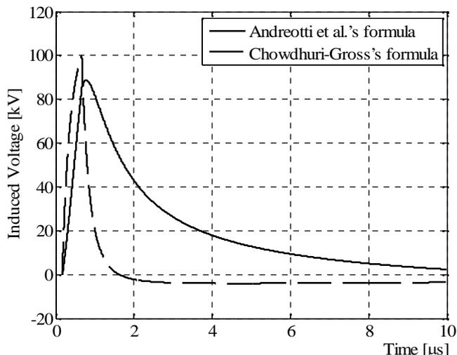
Fig. 5. Comparison between the voltage evaluated at  $x = 0$  by means of Chowdhuri–Gross’s and Andreotti *et al.*’s formulas ( $h = 10$  m,  $d = 50$  m,  $I_0 = 12$  kA,  $s = 0.4$ ,  $t_f = 0.5$   $\mu$ s,  $t_t = 20$   $\mu$ s,  $h_c = 3$  km).
