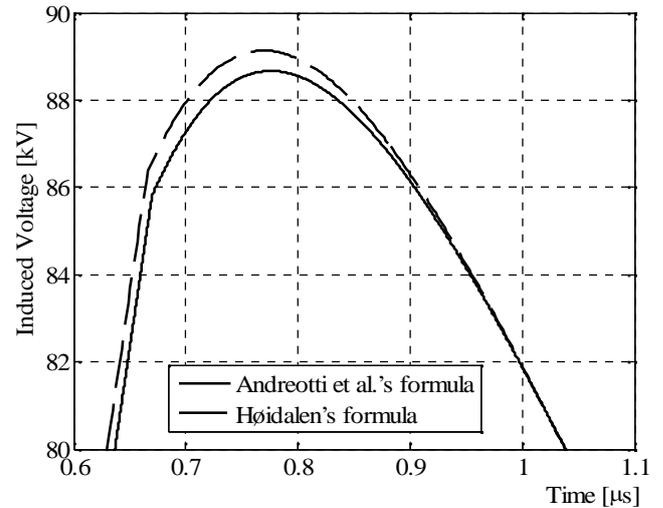
Fig. 13. Comparison between the voltage evaluated at  $x = 0$  by means of Hoidalén's and Andreotti *et al.*'s formulas ( $h = 10$  m,  $d = 50$  m,  $I_0 = 12$  kA,  $\alpha = 0.4$ ,  $t_f = 0.5$   $\mu$ s,  $t_r = 20$   $\mu$ s): magnification of the 0.6–1.1  $\mu$ s time interval.
