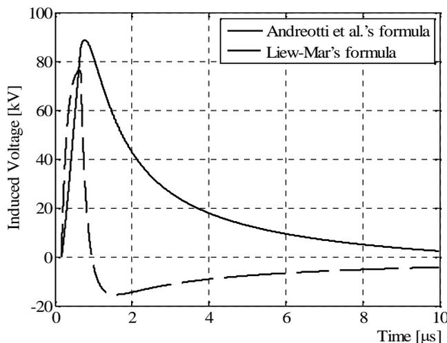
Fig. 9. Comparison between the induced voltage evaluated at  $x = 0$  by means of Liew-Mar’s and Andreotti *et al.*’s formulas ( $h = 10$  m,  $d = 50$  m,  $I_0 = 12$  kA,  $s = 0.4$ ,  $t_f = 0.5$   $\mu$ s,  $t_t = 20$   $\mu$ s,  $h_c = 3$  km).
