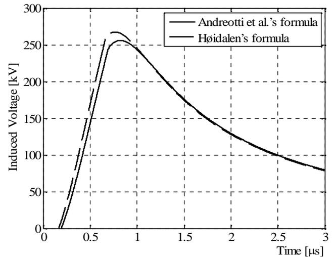
Fig. 14. Comparison between the voltage evaluated at  $x = 0$  by means of Hoidalén's and Andreotti *et al.*'s formulas ( $h = 30$  m,  $d = 50$  m,  $I_0 = 12$  kA,  $\alpha = 0.4$ ,  $t_f = 0.5$   $\mu$ s,  $t_r = 20$   $\mu$ s).
