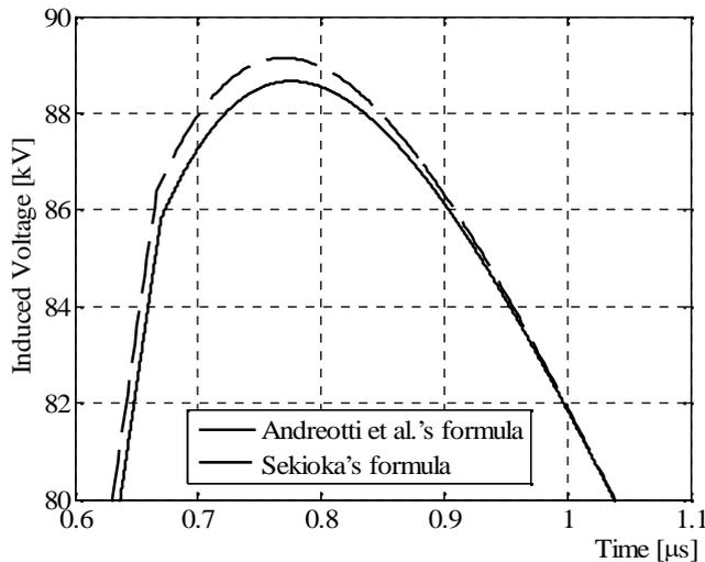
Fig. 11. Comparison between the voltage evaluated at  $x = 0$  by means of Sekioka's and Andreotti *et al.*'s formulas ( $h = 10$  m,  $d = 50$  m,  $I_0 = 12$  kA,  $\alpha = 0.4$ ,  $t_f = 0.5$   $\mu$ s,  $t_r = 20$   $\mu$ s): magnification of the 0.6–1.1  $\mu$ s time interval.
