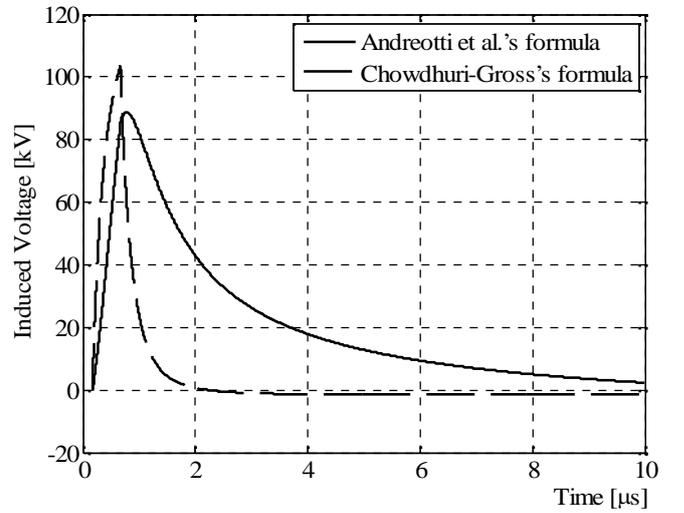
Fig. 3. Comparison between the voltage evaluated at  $x = 0$  by means of Chowdhuri-Gross's and Andreotti *et al.*'s formulas ( $h = 10$  m,  $d = 50$  m,  $I_0 = 12$  kA,  $S = 0.4$ ,  $t_f = 0.5$   $\mu$ s,  $t_t = 20$   $\mu$ s,  $h_c = \infty$ ).
