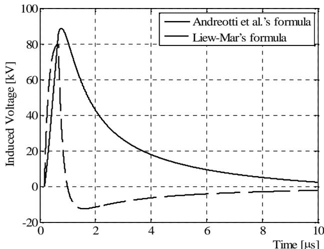
Fig. 7. Comparison between the induced voltage evaluated at  $x = 0$  by means of Liew-Mar’s and Andreotti *et al.*’s formulas ( $h = 10$  m,  $d = 50$  m,  $I_0 = 12$  kA,  $s = 0.4$ ,  $t_f = 0.5$   $\mu$ s,  $t_t = 20$   $\mu$ s,  $h_c = 3$  km).
