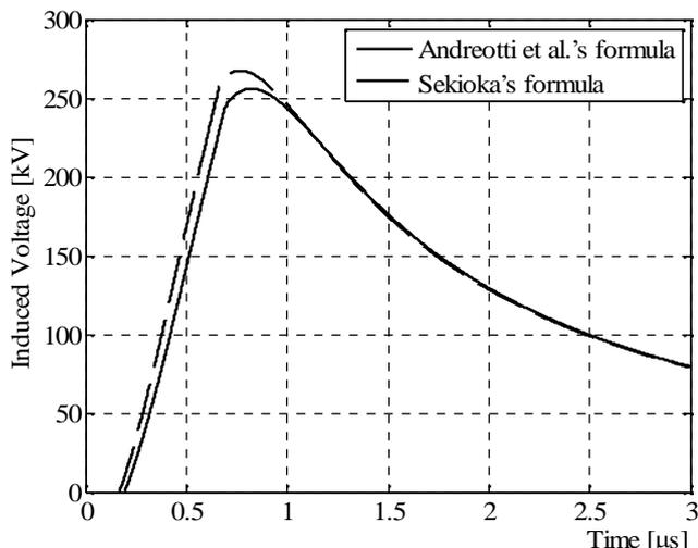
Fig. 12. Comparison between the voltage evaluated at  $x = 0$  by means of Sekioka's and Andreotti *et al.*'s formulas ( $h = 30$  m,  $d = 50$  m,  $I_0 = 12$  kA,  $\alpha = 0.4$ ,  $t_f = 0.5$   $\mu$ s,  $t_r = 20$   $\mu$ s).
