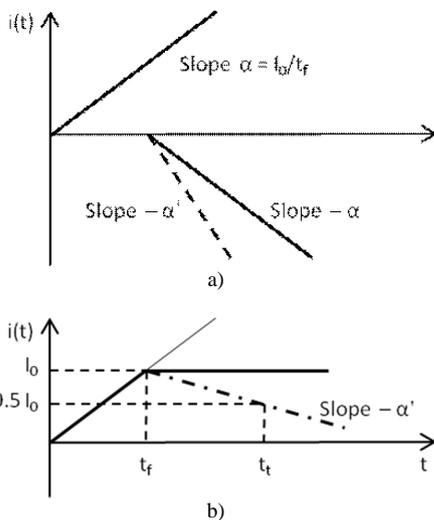
Fig. 2. Current waveshapes: ramp with constant or drooping tails.
