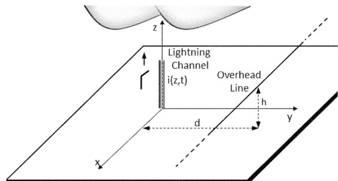
Fig. 1. A typical configuration for lightning-induced voltage calculations.
