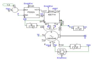
Fig. 4. PSCAD model of CHP generator.
