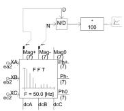
Fig. 5. Unbalance measuring scheme in PSCAD.
