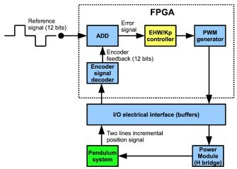
Fig. 10. Simplified FPGA content diagram.
