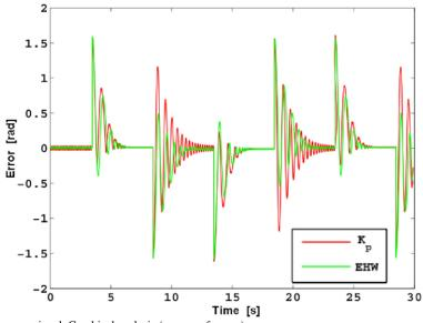
Fig. 12. Temporal response of the error signal. Graphical analysis (square reference).
