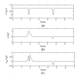
Fig. 8. (a)  $\Lambda(\omega_0 t)$  (b)  $\alpha(\omega_0 t)$  (c)  $\Lambda_{eff}(\omega_0 t)$  for ring oscillator.
