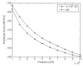
Fig. 10. Amplitude noises calculated by HB and (6) for 19-stage ring oscillator.
