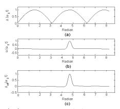
Fig. 7. (a)  $\Lambda(\omega_0 t)$ ; (b)  $\alpha(\omega_0 t)$ ; (c)  $\Lambda_{eff}(\omega_0 t)$  for Colpitts oscillator.
