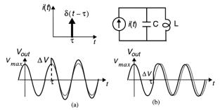
Fig. 1. Time domain response of an oscillator (a) impulse is injected at the peak (b) impulse is injected at the zero crossing point.
