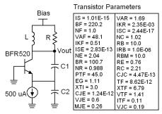
Fig. 3. The Colpitts oscillator.
