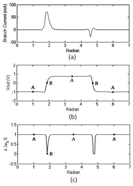
Fig. 6. (a) Branch current (b) output voltage (c) A-ISF (ring oscillator).
