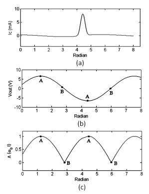
Fig. 4. (a) Transistor current (b) output voltage (c) A-ISF (Colpitts oscillator, R=10k $\Omega$ , L=200nH, C1=40pF, C2=200pF, f=62MHz).
