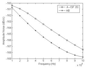
Fig. 9. Amplitude noises calculated by HB and (6) for Colpitts oscillator with R=10k $\Omega$ , L=200nH, C1=40pF, C2=200pF.
