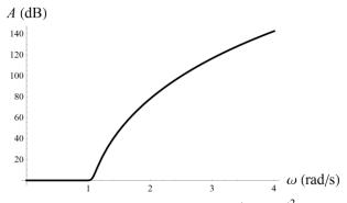
Fig. 2. Attenuation of the filter  $A = -10\log_{10} |H_n(j\omega)|^2$  in dB for n = 10, v = 0.5,  $\rho = 0.1$ .
