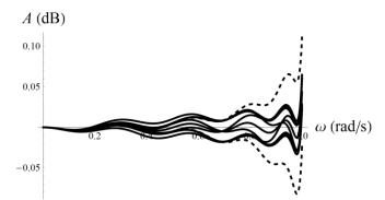
Fig. 7. Overall attenuation for  $\pm 0.2\%$  tolerances of the pole magnitudes (biquad with critical Q factor - dashed lines, other biquads - solid line).
