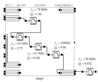
Fig. 4. Implementation with programmable chips.
