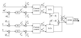
Fig. 1. DFIG's double SRF control structure under unbalanced grid voltage.
