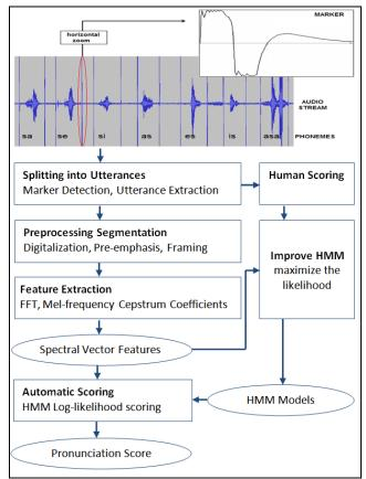
Fig. 1. The architecture of automatic pronunciation scoring system
