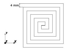
Fig. 1. Designed square spiral antenna.
