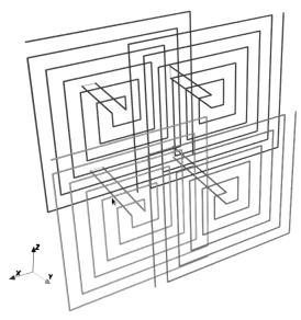
Fig. 2. Overlapping wire antennas.
