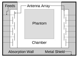
Fig. 3. Construction of the proposed chamber.
