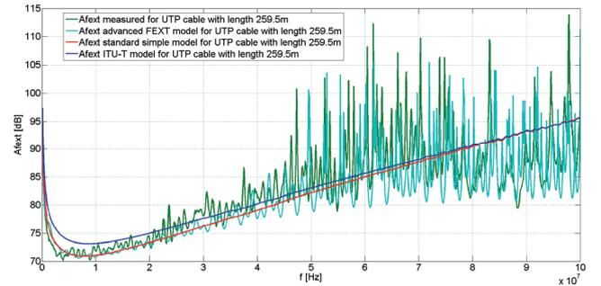
Fig. 4. The comparison between measured results, models and the advanced FEXT model for the length of a cable 259.5 m
