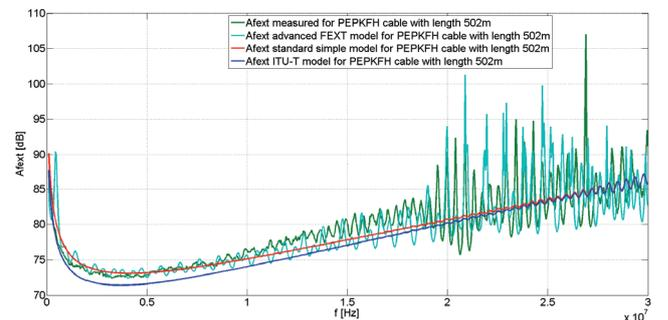
Fig. 6. The advanced FEXT model, both standard models and measured characteristic for PEPKFH cable
