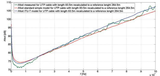
**Fig. 3.** Measured FEXT attenuation, simple FEXT model and ITU-T model for a UTP cable with length 83.5 m recalculated to a ref. length 264.5 m
