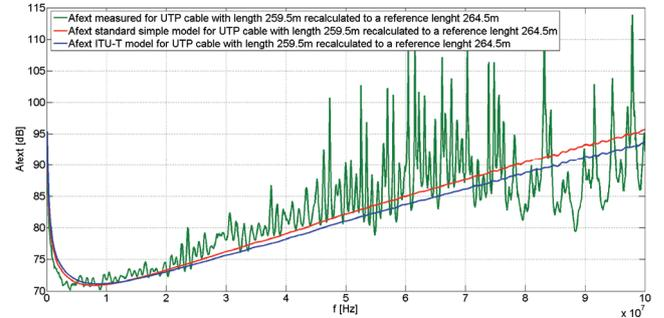
**Fig. 1.** Measured FEXT attenuation, simple FEXT model and ITU-T model for a UTP cable with length 259.5 m recalculated to a ref. length 264.5 m
