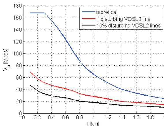
Fig. 9. Transmission rate VDSL2 line, frequency band plan B8-12 for downstream direction
