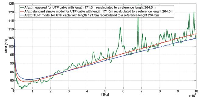
**Fig. 2.** Measured FEXT attenuation, simple FEXT model and ITU-T model for a UTP cable with length 171.5 m recalculated to a ref. length 264.5 m
