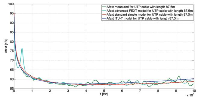
Fig. 5. The comparison between measured results, models and the advanced FEXT model for the length of a cable 87.5 m
