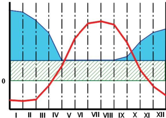
Fig. 2. Outdoor temperature and heat consumption during a year
