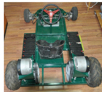
Fig. 1. Kart with both motors and battery packs
