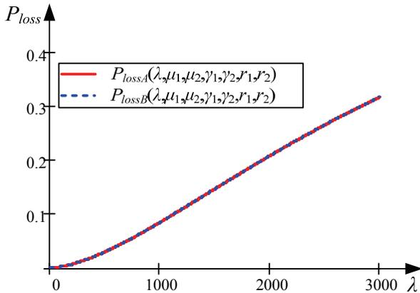
**Fig. 4.** Results of data packet transmission loss obtained by the means of detailed states Markov model –  $P_{lossA}$  and the macro states Markov model –  $P_{lossB}$  as a function of data packet arrival rate  $\lambda$ , when  $\mu_1=\mu_2=\mu=2000$  pack/s,  $\gamma_1=1/5000$  [hours<sup>-1</sup>],  $\gamma_2=1/1000$  [hours<sup>-1</sup>],  $r_1=r_2=1/24$ [hours<sup>-1</sup>]
