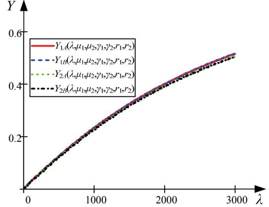
**Fig. 5.** Results of data packet transmission channels utilization obtained by the means of detailed states Markov model –  $Y_{1A}, Y_{2A}$ , and the macro states Markov model –  $Y_{1B}, Y_{2B}$  as a function of data packet arrival rate  $\lambda$ , when  $\mu_1=\mu_2=\mu=2000$  pack/s,  $\gamma_1=1/5000$  [hours<sup>-1</sup>],  $\gamma_2=1/1000$  [hours<sup>-1</sup>],  $r_1=r_2=1/24$ [hours<sup>-1</sup>]
