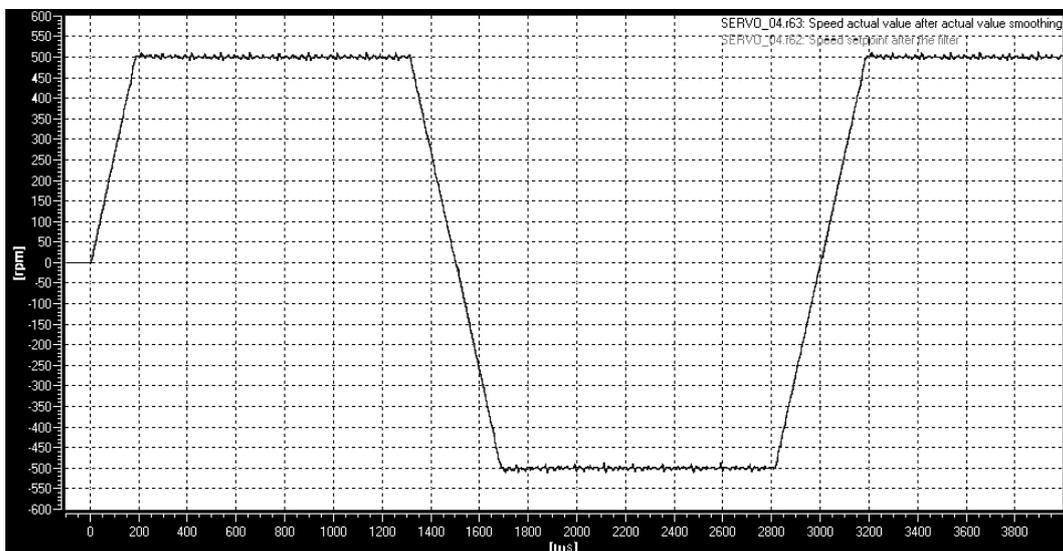
Fig. 5. Time response of the speed of the 1<sup>st</sup> axis drive to changes in speed reference value with linearly increasing signal. Scale: vertical axis – speed scale <-600, 600> rpm, horizontal axis – time scale 3900 ms.
