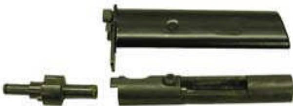
Fig. 2. CO<sub>2</sub> gas recoil system for M16
