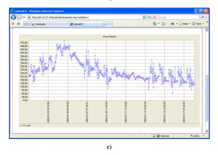
**Fig. 6.** RIS software user interface windows: remote control of heating system parameters (a), heating system parameters data log over the selected period (b) and analysis window of heat energy consumption over the selected period of time (c)
