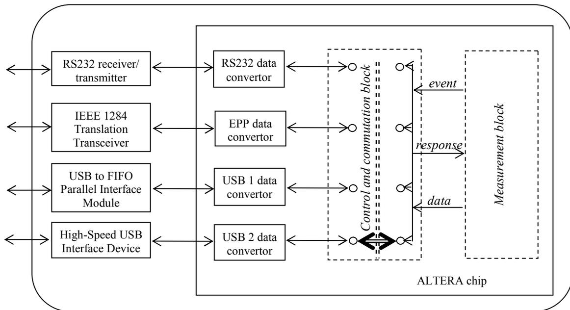
**Fig. 3.** Schematic block diagram of measurement hardware
