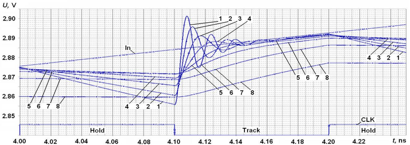
**Fig. 2.** 8-bit THC time diagrams, when parasitic inductances  $L = 0.2$  nH. Here CLK – 5 GHz clock signal, In – analog input signal, 1 – THC output signal, when  $\tau = 15$  fs, 2 –  $\tau = 30$  fs, 3 –  $\tau = 60$  fs, 4 –  $\tau = 120$  fs, 5 –  $\tau = 250$  fs, 6 –  $\tau = 0.5$  ps, 7 –  $\tau = 1$  ps, 8 –  $\tau = 2$  ps
