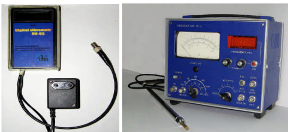
Fig. 4. Measuring vibrations instrument (a) and cavitometr (b)
