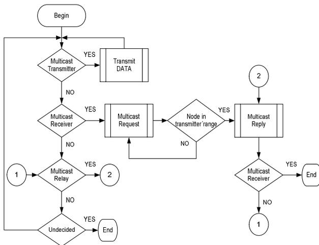
**Fig. 2.** Flow diagram of the ToMuRo algorithm
