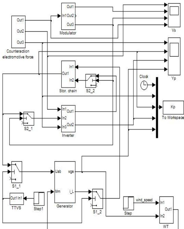
Fig. 3. Mathematical model for the WT’s power conversion
