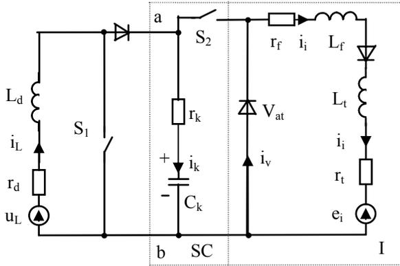
Fig. 2. Equivalent scheme of the power converter
