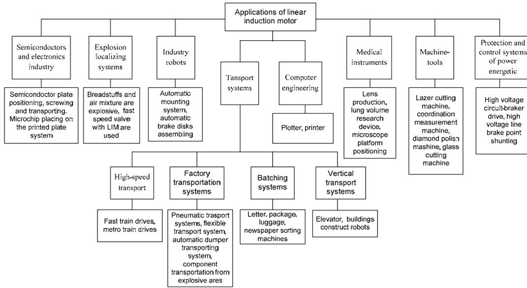
Fig. 4. Areas of application of linear induction drives
