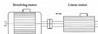
Fig. 3. Combination of linear and revolving drive
