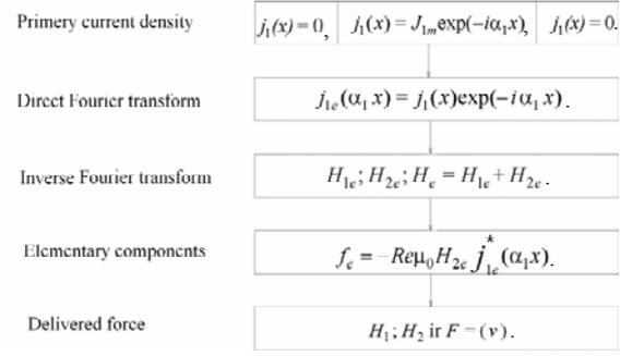
Fig. 5. Algorithm for calculation of LIM characteristics
