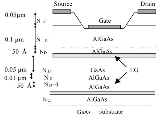
Fig. 1. Submicron HEMT structure with two potential wells
