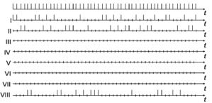
Fig. 4. Decomposition of periodic sampling point process with jitter
