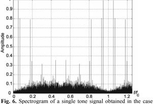
**Fig. 6.** Spectrogram of a single tone signal obtained in the case periodic sampling with jitter
