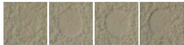
Fig. 2. Footprints of the probe tip when the cathode is moved with different speeds
