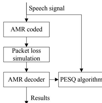
Fig. 3. Simulation scheme
