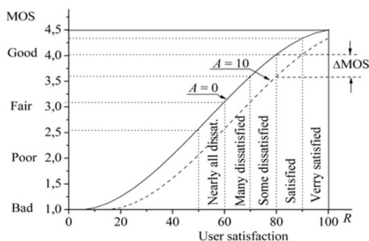
**Fig. 2.** Application of E-model for user satisfaction estimation
