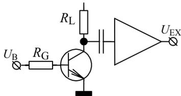
Fig. 2. Noise measurement circuit without common feedback
