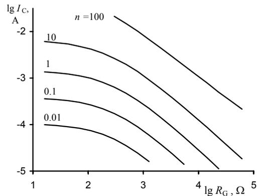
**Fig. 8.** Ratio ( $n$ ) of base noise  $S_\pi$  to collector noise  $S_o$  in total output current noise as a function of collector current  $I_C$  and source resistance  $R_G$
