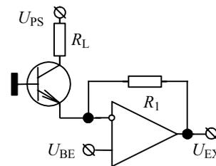
Fig. 5. Noise measurement circuit with common feedback
