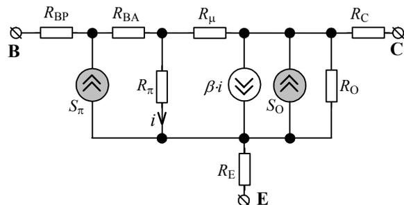
Fig. 1. BJT model with low frequency noise sources
