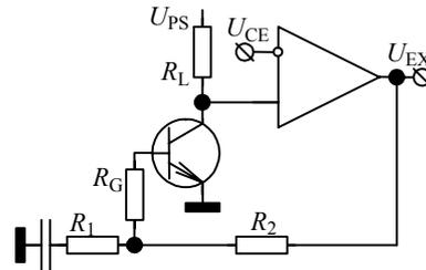
Fig. 4. Noise measurement circuit with common feedback
