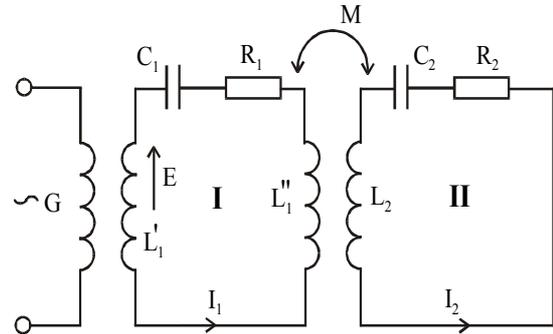
Fig. 4. The equivalent circuit of HM
