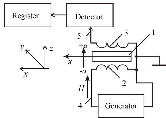
Fig. 1. The experimental device of Helicon Maser
